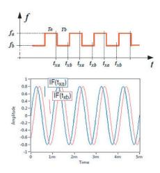
It is important to mention that by both FMCW and FSK techniques it is possible to measure distance, however FMCW is usually used to measure distance of stationary objects, while FSK is used for moving objects.
