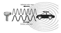
A person can be detected at a distance of 12 meters even with smallest standard modules. Many of the plastic materials are more or less transparent for microwave radiation. Therefore the sensor module can easily be hidden behind a plastic panel which is a huge advantage for the outdoor design of the final product compared to pyroelectric detectors, which need a Fresnel lens for proper operation.
